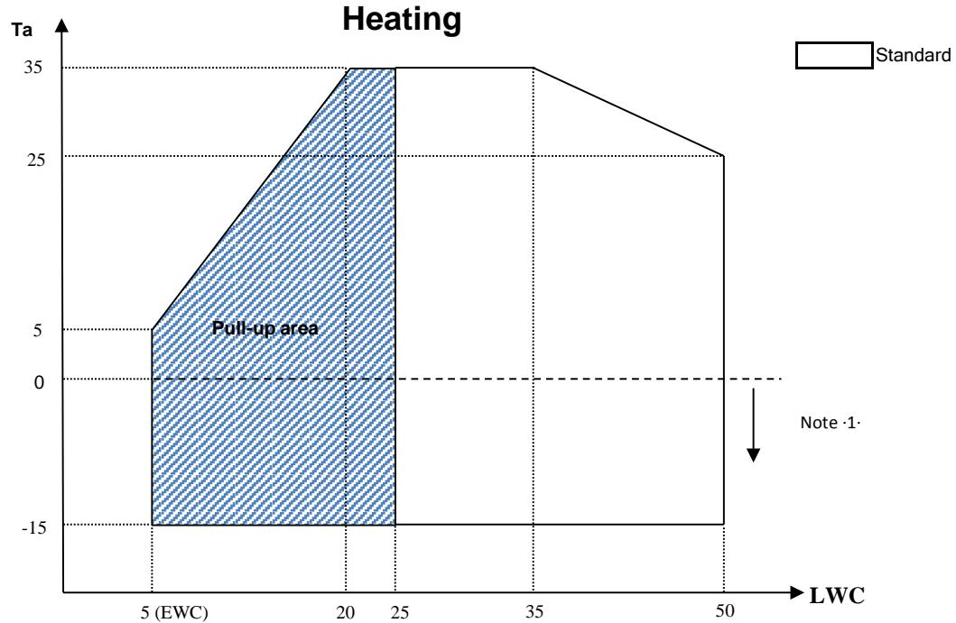
**Symbols**Ta: Ambient temperature [ $^{\circ}\text{C DB}$ ]LWC: Leaving water condenser temperature [ $^{\circ}\text{C}$ ]EWC: Entering water condenser temperature [ $^{\circ}\text{C}$ ]**Note ·1·**
