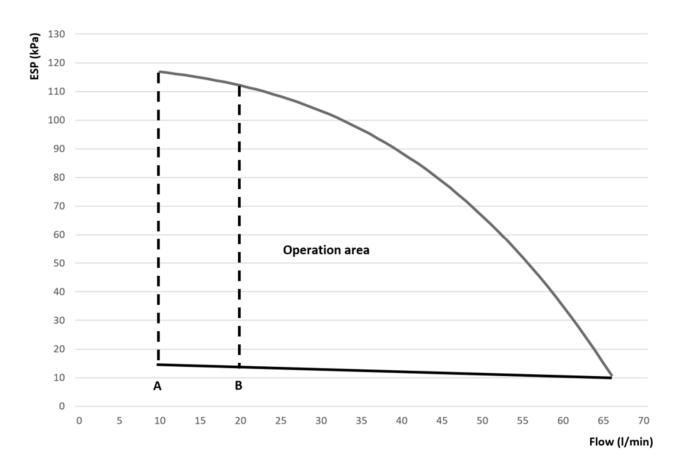
ESP = External static pressure [kPa] Space heating/cooling circuit
