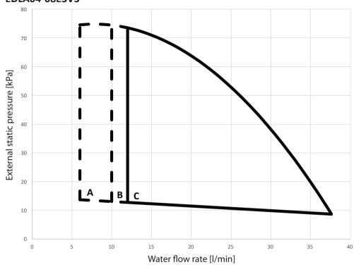
A = Minimum water flow rate during normal operation
