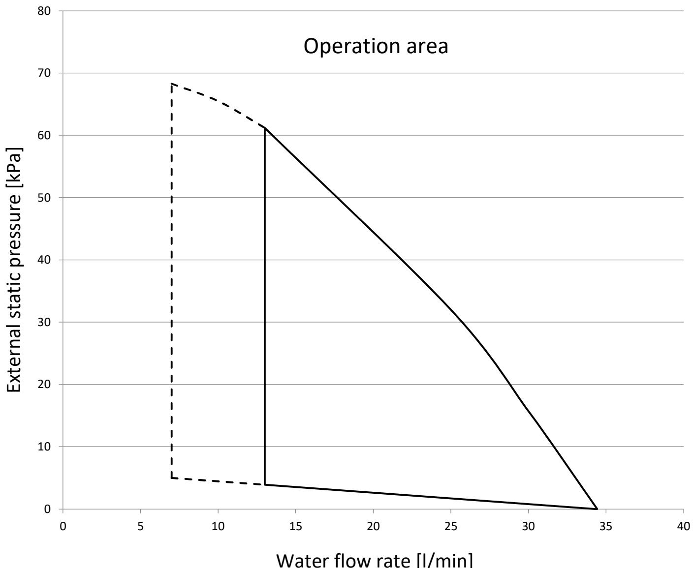
Operation area is extended to lower flow rates only in case the unit operates with heat pump only.
