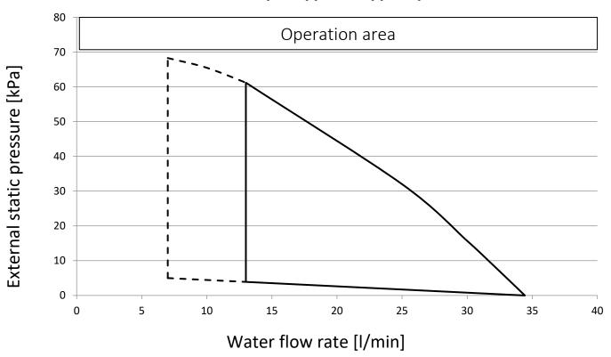
Operation area is extended to lower flow rates only in case the unit operates with heat pump only.
