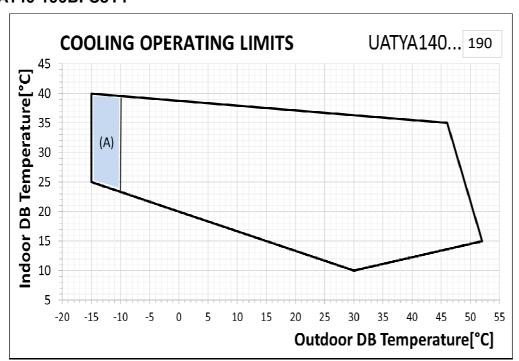
Outdoor DB Temperature [°C]: Outdoor air temperature that strikes the condensing coil (dry bulb). Indoor DB Temperature [°C]: Indoor air temperature that strikes the evaporating coil (dry bulb).
