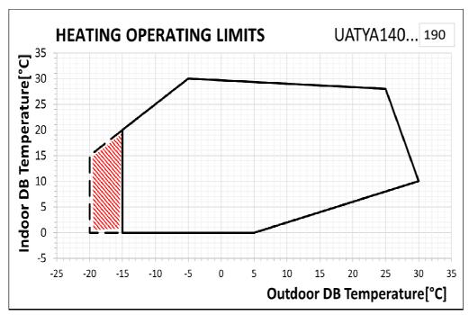
**Outdoor DB Temperature** [°C]: Outdoor air temperature that strikes the evaporating coil (dry bulb). **Indoor DB Temperature** [°C]: Indoor air temperature that strikes the condensing coil (dry bulb).
