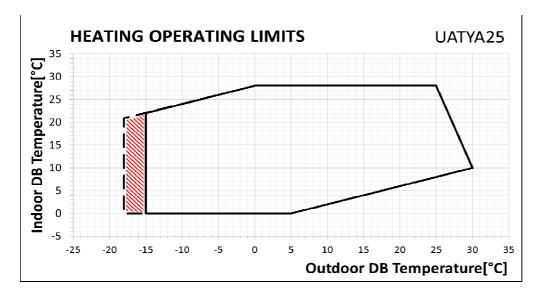
**Outdoor DB Temperature** [°C]: Outdoor air temperature that strikes the evaporating coil (dry bulb). **Indoor DB Temperature** [°C]: Indoor air temperature that strikes the condensing coil (dry bulb).
