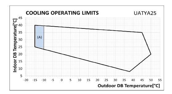
**Outdoor DB Temperature** [°C]: Outdoor air temperature that strikes the condensing coil (dry bulb). **Indoor DB Temperature** [°C]: Indoor air temperature that strikes the evaporating coil (dry bulb).
