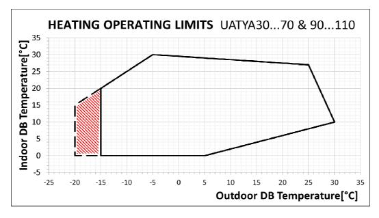
Outdoor DB Temperature [°C]: Outdoor air temperature that strikes the evaporating coil (dry bulb). Indoor DB Temperature [°C]: Indoor air temperature that strikes the condensing coil (dry bulb).
