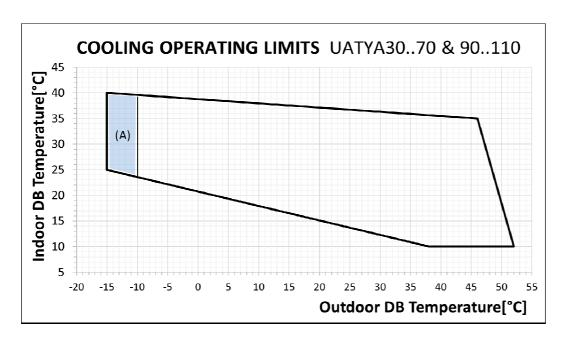
Outdoor DB Temperature [°C]: Outdoor air temperature that strikes the condensing coil (dry bulb). Indoor DB Temperature [°C]: Indoor air temperature that strikes the evaporating coil (dry bulb).
