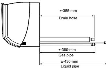
Dimensions of fully opened front panel
