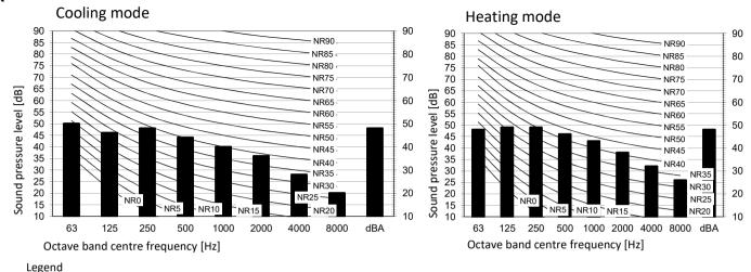
dBA = A-weighted sound pressure level (A scale according to IEC).
