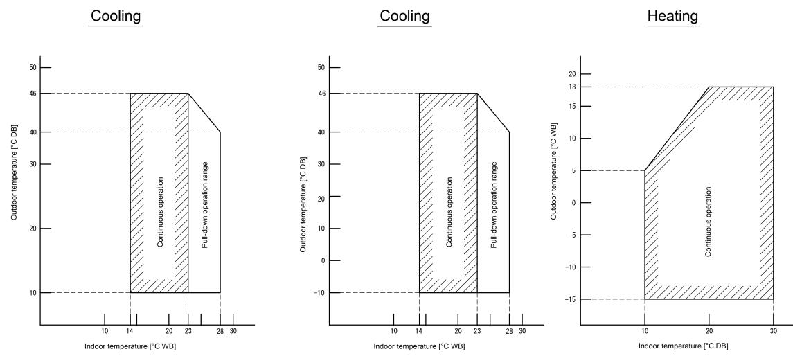
The values above are for connecting with the following indoor unit types: The values above are for connecting with the following indoor unit types:
