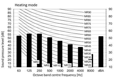
Legend dBA = A-weighted sound pressure level (A scale according to IEC).
