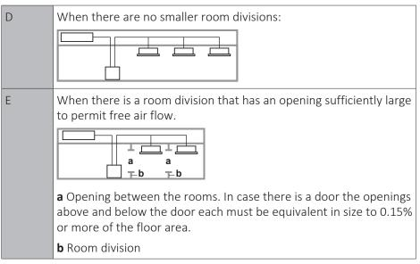
3 Calculate the refrigerant density using the results of the calculations in steps 1 and 2 above. If the result of the above calculation exceeds the maximum concentration level, a ventilation opening to the adjacent room shall be made.
