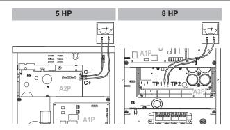
To prevent damaging the PCB, touch a non-coated metal part to eliminate static electricity before pulling out or plugging in connectors.
