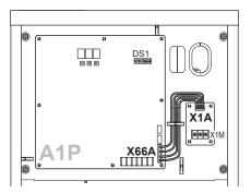
Connect the cool/heat selector switch. Tightening torque X1M (A/B/C): 0.53~0.63 N•m
