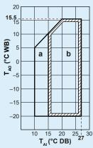
$\mathbf{a}$ : Warming up operation range;  $\mathbf{b}$ : Heating operation range;  $\mathbf{T}_{AI}$ : Ambient indoor temperature;  $\mathbf{T}_{AO}$ : Ambient outdoor temperature
