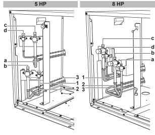
a Liquid line (circuit 1: to heat exchanger unit)
