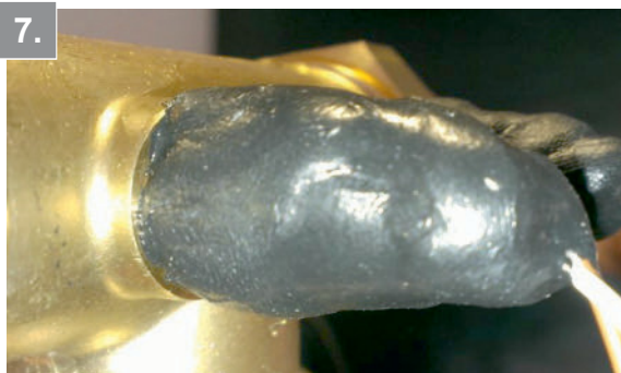
7. after 24h the material has created a shining layer
