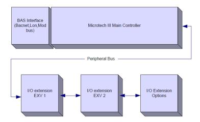
All boards are supplied from a common 24 Vac source. Extension boards can be directly powered by the Unit Controller. All boards can be also supplied by a 24Vdc source.
