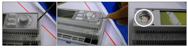
Be careful to avoid damages to the plastic cover. The new battery shall be placed in the proper battery holder which is highlighted in the picture, respecting the polarities indicated into the holder itself.
