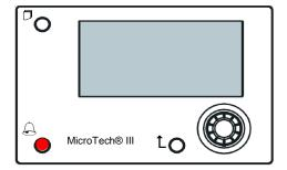
The Remote HMI can be extended up to 700 m using the process bus connection available on the UC. With a daisy-chain connection as below, a single HMI can be connected to up to 8 units. Refer to the specific HMI manual for details.
