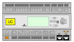
The keypad/display (A) consists of a 5-line by 22 character display. The function of the three buttons (B) is described below:
